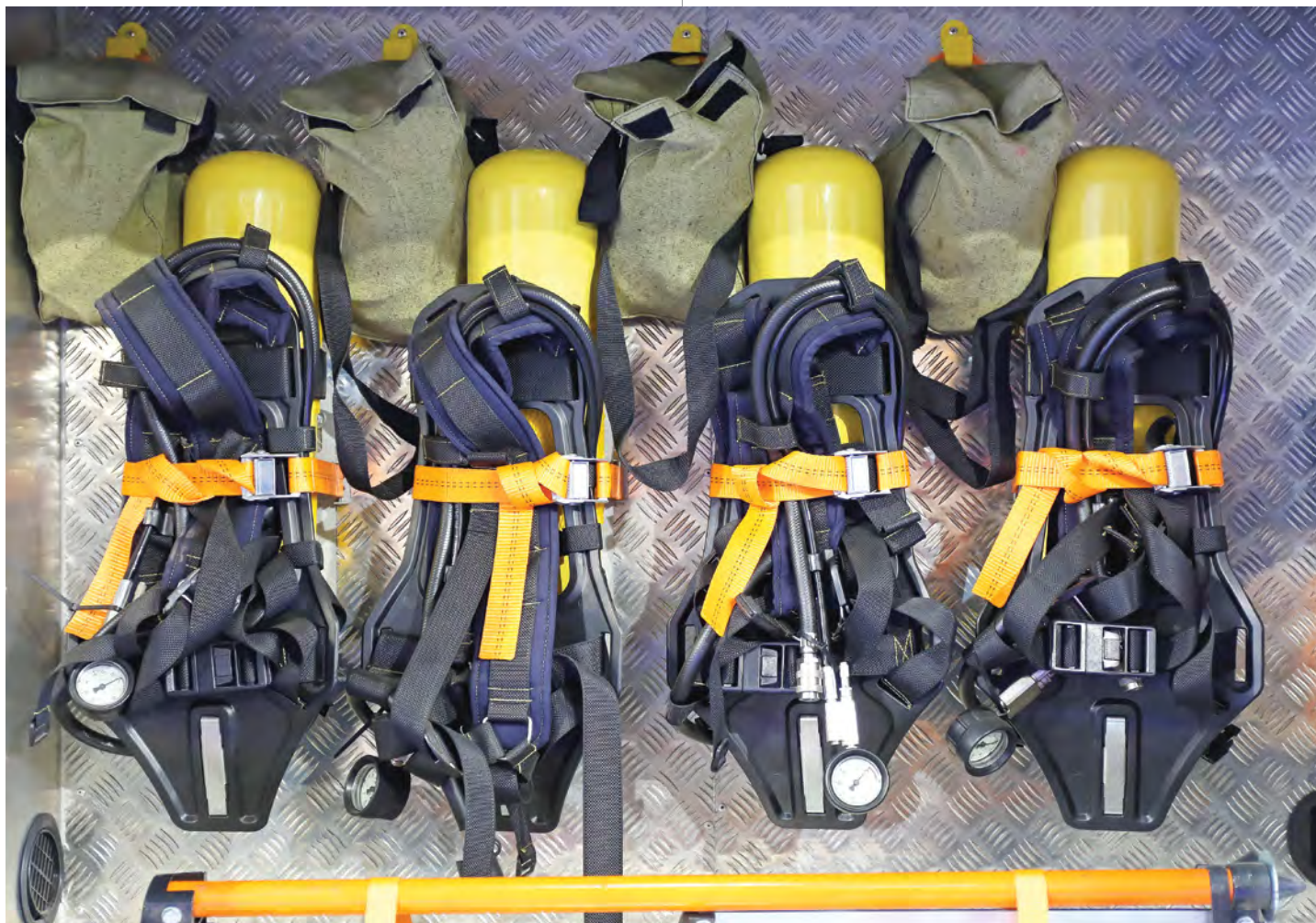
ABOVE: SCBAs and turnouts should have their own compartment away from the cab.
