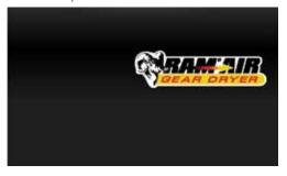
Note: If the unit is sitting idle for some time, the screen may show a screensaver with a floating Ram Air logo as shown above. Touching the LCD Panel brings the GUI back.
