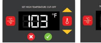
Press the form once to show the current temperature sensor reading. The temperature reading is indicated by a thermometer icon next to the reading. If it shows a temperature value as illustrated above, then the thermostat is working properly.
