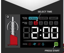
STEP SEVEN Monitor drying progress-checking hard-to-dry areas (armpits, fingertips, etc.). Adjust dry time until gear is fully dry.
